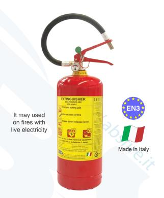
The basic components of dry powder are ammonium phosphate and ammonium sulphate with special silicones additives enabling easy flow discharge and avoiding any caking process.
